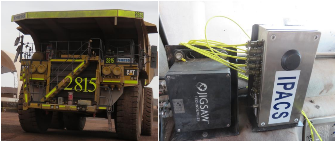
Figure 7: Installation of IPACS sensors and data acquisition system on a Thies Caterpillar 793D truck at Oz Minerals Prominent Hill mine
