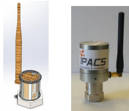
Figure 10 - Prototype wireless sensor designed and developed as part of the project
