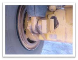
Sensor installed on the POS3 wheel hub
