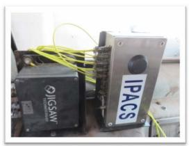
Installation of the IPACS remote monitoring box inside the driver cabin
